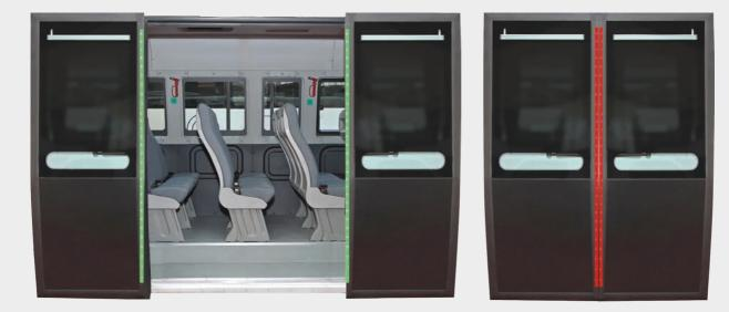
Green signal illumination: *SensIQ signal* shows that doors are open or in the process of opening
